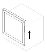
Open the door of the beverage cabinet and detach the glass door with tremendous care.
