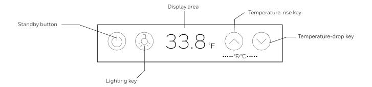
When powering on the cooler for the first time, the display screen will display in full for 3 seconds and the start-up tone will ring, and then the display will enter a normal running state.
