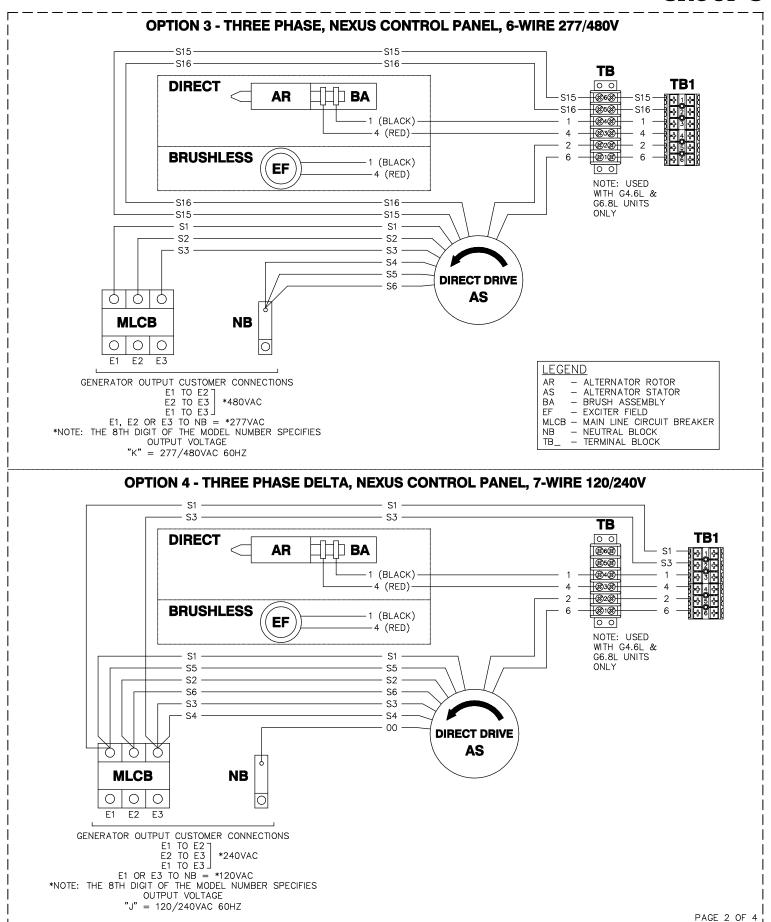
WIRING - DIAGRAM NEXUS CPL ALTERNATOR DRAWING #: 0H6342
