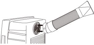
4 Connect the window bracket to the opposite end of the plastic hose. Ensure that all connections are tight and installed properly.
