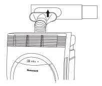
(5) Connect the window bracket to the window.
